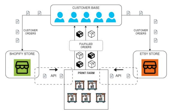
Customers send orders to a Shopify or Etsy store. The stores are linked to a 3D printing service provider by an API which allows specific orders to be routed to the print farm. The parts are produced and packaged at the print farm and delivered directly to customers.
